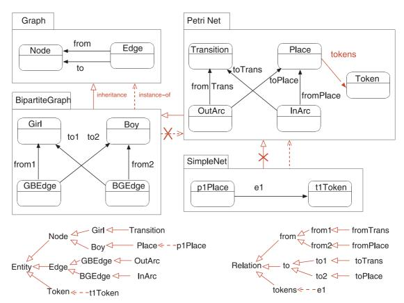
Fig. 6. Defining the structure of Petri Nets
