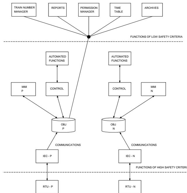
Fig.2. Block diagram of the WS software
