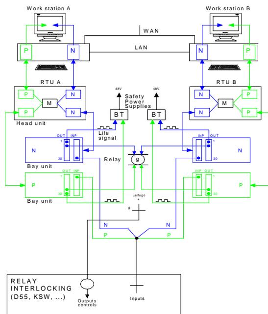
Fig. 1. Hardware architecture of the electronic control desk
