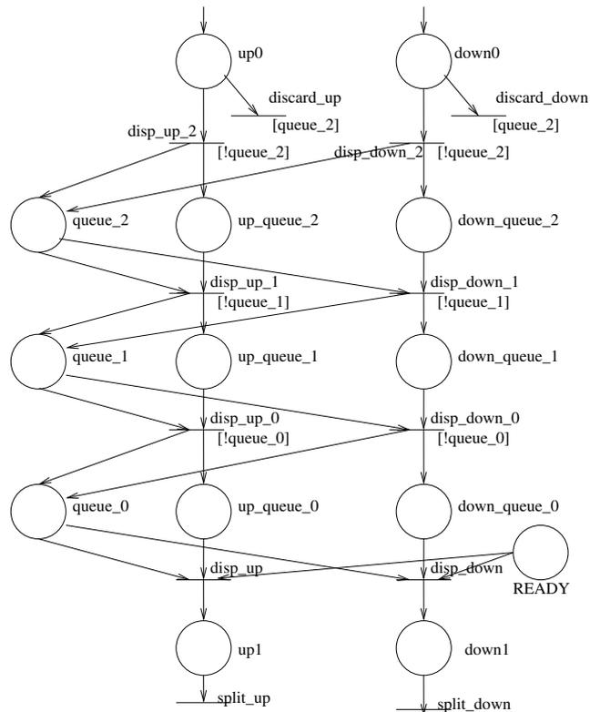
FIGURE 2. SRN pattern of a FIFO event dispatcher.
