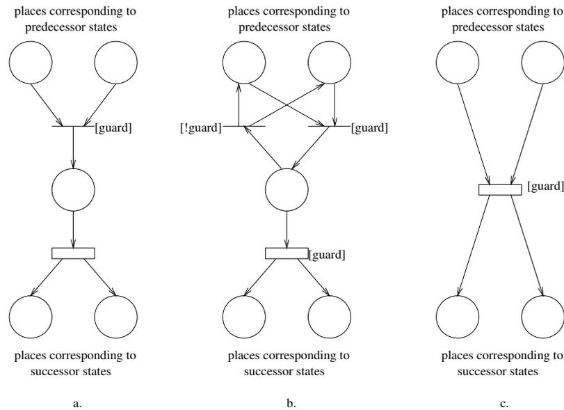
FIGURE 6. Models for combining guards and timing.
