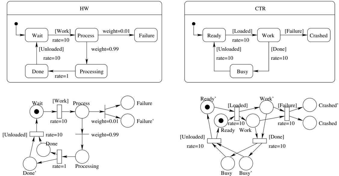
FIGURE 9. GSC model and the corresponding SRN model of the press.
