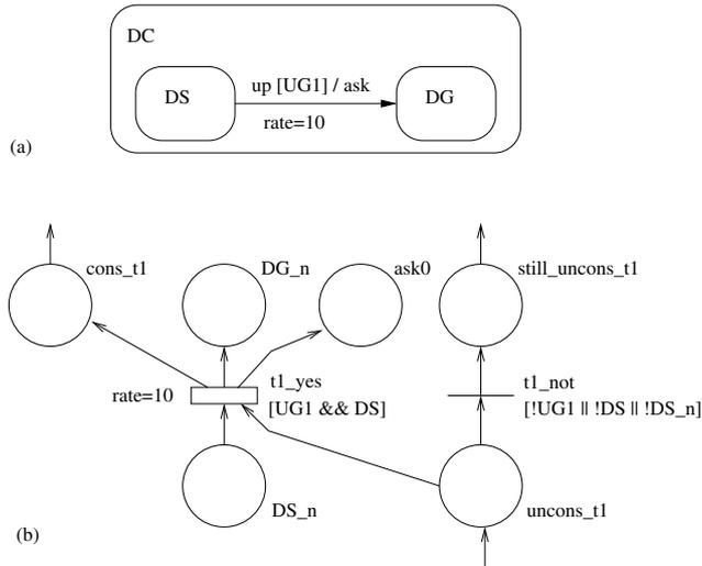
**FIGURE 4.** A simple UML transition (a) and the corresponding SRN pattern (b).
